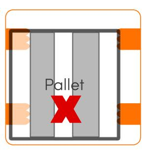
Your IBC pallet should be centrally located on the IBC bund support columns.
