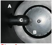
Step 4 Pull the mini basket filter through to expose the filter.
