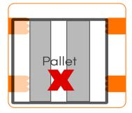
Your IBC pallet should be centrally located on the IBC bund support columns.
